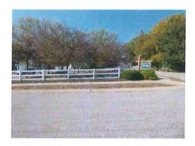
The Sweetbriar Entrance to the west consists of a composite sign 3 1/2' x 2 1/2', engraved and painted, and mounted to a wooden post 7' 6" in height. Additionally there is a 3 rail white pvc fence 3 1/2' in height and 72' in length.
