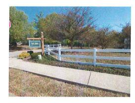
The Sweetbriar Entrance to the west consists of a composite sign 3 1/2' x 2 1/2', engraved and painted, and mounted to a wooden post 7' 6" in height. Additionally there is a 3 rail white plastic fence 3 1/2' in height and 88' in length.
